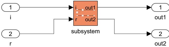
(a) The root subsystem view of the model. A subsystem is shown in **apricot**, while its implementation content is hidden. The implementation content (*c.f.* Figure 1b) is only hinted at on the subsystem symbol.
